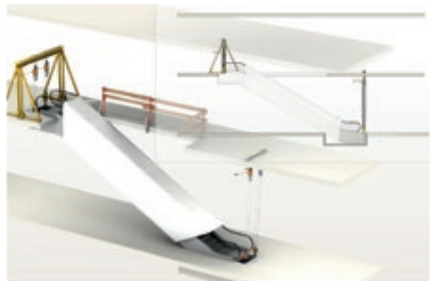
Figure 8.5 Installation using a lifting frame
